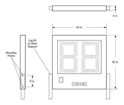
If you wish to attach your play clock displays to a different support structure, you may take advantage of the mounting plates included in the cabinets. These plates have tapped holes, spaced nine inches center-to-center, along the sides of each cabinet. The tapped holes accept 1/2-inch-13 threaded bolts. For Model LX3024, support brackets or posts would need to be positioned 42 inches apart (inside spacing) to provide room for the cabinet.
